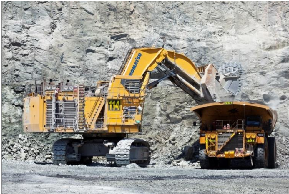
Figure 6 - Fimiston Pit, PC8000 face shovel loading a CAT793 truck
