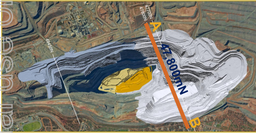
ABOVE: Plan view of Fimiston cutback stages with the location of the 47,800mN cross section shown
