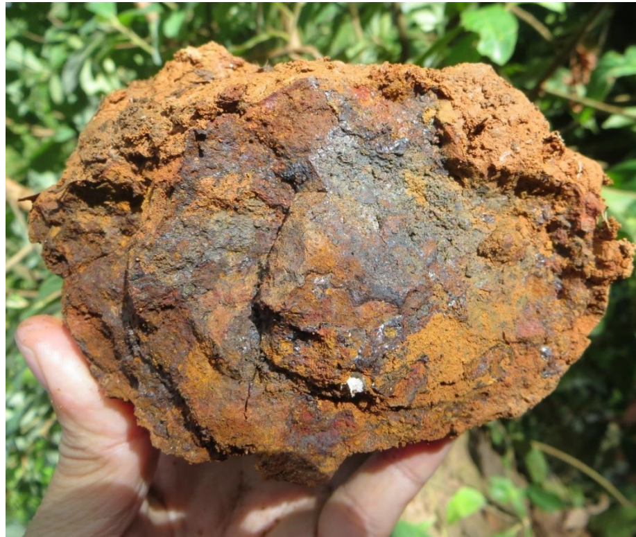
Figure 1: Gossan float in the overburden at trench BCH20-03
