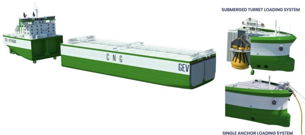
Figure 4: CNG Optimum ship equipped with examples of offshore loading systems
