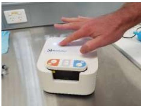
The Felix device incorporates a simple automated process that efficiently separates sperm in around 6 minutes. This is a marked improvement on the current sperm preparation techniques, density gradient centrifugation ("DGC") and "Swim up", currently used in IVF clinics. These techniques are time consuming (each taking 30 to 40 minutes), laborious, and heavily dependent on operator expertise.
