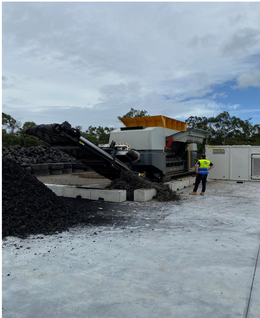
Image 1: Pearl's first stage waste tyre shredding process. Tyres are placed whole in the top of the above shredder and shredded down to 80mm with all steel and nylon left in, ready for Thermal desorption processing. Source: Company
