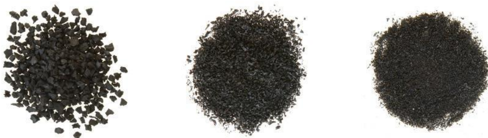
Image 1: Rubber crumb comes in various sizes depending on commercial applications. Finer sizes (far right) is 30 mesh and typically used in asphalt. Far left image is 2mm sizing for sporting and rubber moulds, with the image in the middle 10 mesh.
