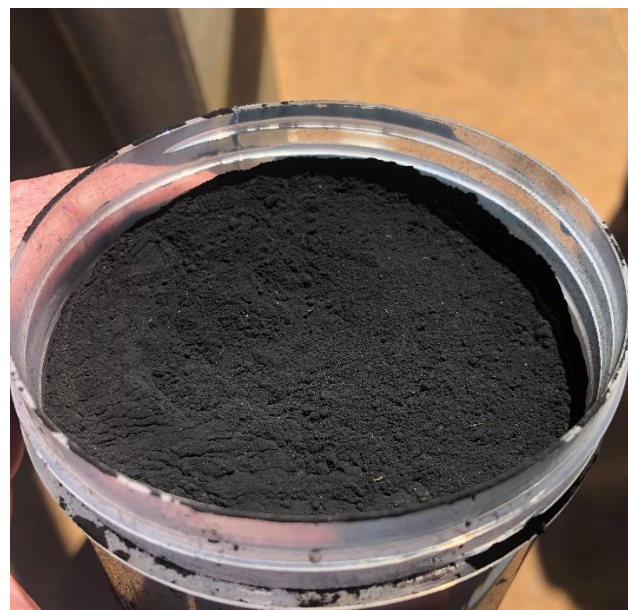
Image 2: Pearl’s carbon char powder. The Company’s carbon char has similar properties to crumb rubber with the carbon char having less impurities given it has been exposed the Pearl’s thermal desorption heat process. Source: Company
