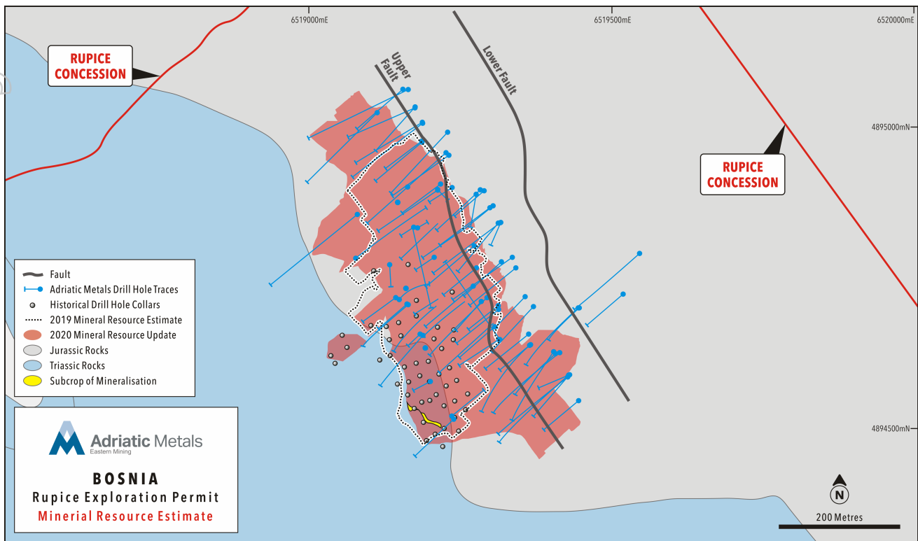
Figure 1 – Plan View of the New Ore Block Model Outline of Rupice vs 2019 Ore Block Model
