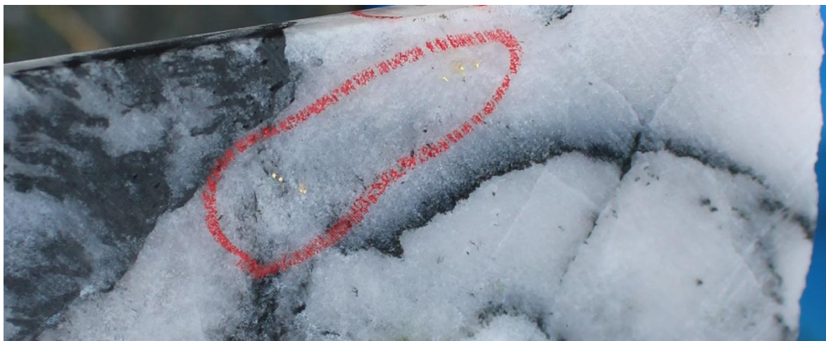
Figure 11: Vein 11 Footwall discovery: AUDD0019: 1.6m @ 19.6 g/t gold from 372m (including 0.5m @ 59.5 g/t gold from 372.35) in AUDD0019. Detail of quartz-tourmaline-gold vein. View of approximately 5cm length of halved NQ core.
