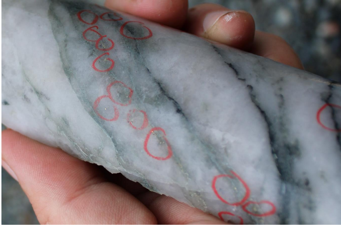
Figure 7: Vein 5 Extension discovery: AUDD0017: 0.6m @ 99.4 g/t gold from 167.4m in AUDD0017 (including 0.3m @ 181.0 g/t gold from 167.4m). 30cm quartz-tourmaline-gold shear vein in high-strain, sericite-ankerite altered basalts with multiple 0.5-1cm shear veins within fabric. NQ core, diameter 47.6mm.
