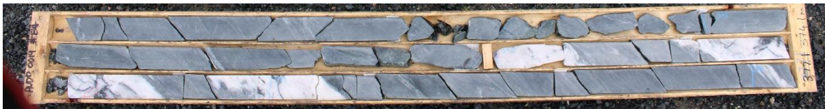
Figure 10: Vein 11 Footwall discovery: AUDD0019: 1.6m @ 19.6 g/t gold from 372m (including 0.5m @ 59.5 g/t gold from 372.35) in AUDD0019. Multiple 20 to 30cm quartz-tourmaline-gold shear veins and quartz-ankerite pyrite extension veins in moderate-strain, sericite-ankerite altered basalts with multiple 0.5-1cm shear veins within fabric.
