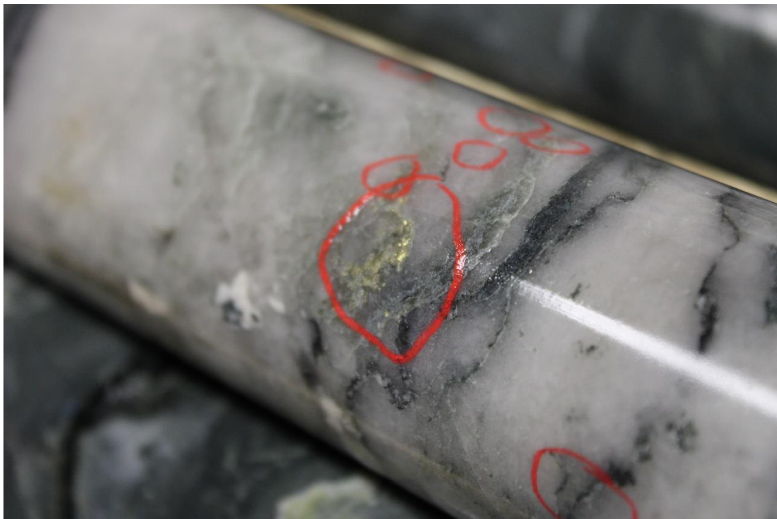
Figure 1: Vein 5 Extension: Close up of new interval outside of Resource Estimate. AUDD0017: Detail of interval grading 0.3m @ 181.0g/t gold from 167.4m (within 0.6m @ 99.4g/t gold from 167.4).
