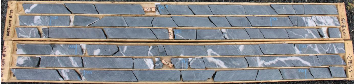
Figure 9: Vein 11 Extension discovery: AUDD0019: 4.85m @ 4.4 g/t gold from 350.15m in AUDD0019. Multiple 1- 15cm quartz-tourmaline-gold shear veins and quartz-ankerite pyrite extension veins in moderate-strain, sericite-ankerite altered basalts with multiple 0.5-1cm shear veins within fabric.
