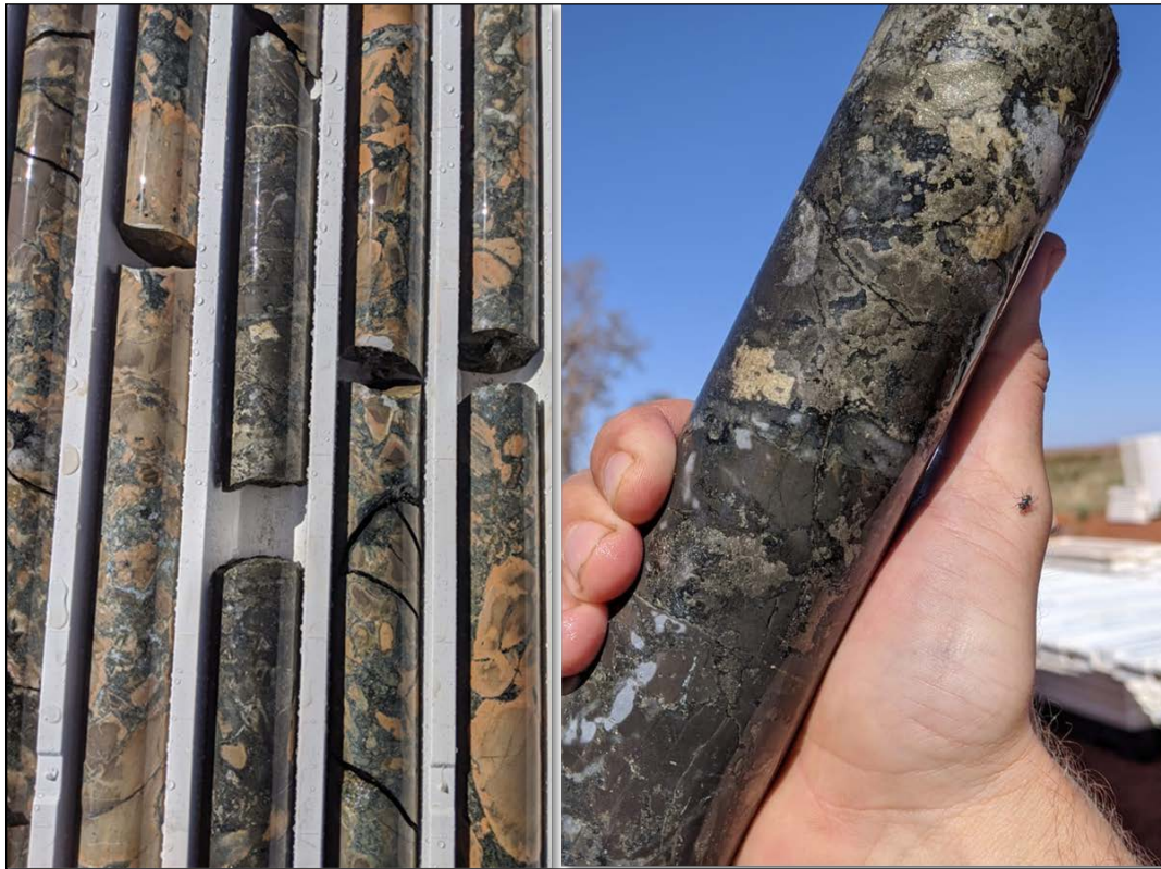
Photos 1&2 ETG0203. Photo 1 (~185-190m) Brecciated and altered sediments containing disseminated and blebby sulphides. Photo 2 (~187m) Coarse euhedral pyrite and fine pyrite alteration within silicified and brecciated sediment. Importantly, the sulphide mineralisation in ETG0203 has a lower chargeability response than the Elsa Prospect.
