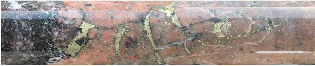
Figure 2. Fracture associated Chalcopyrite mineralisation within albite alteration zones – HMSHDD002, 54.9m
