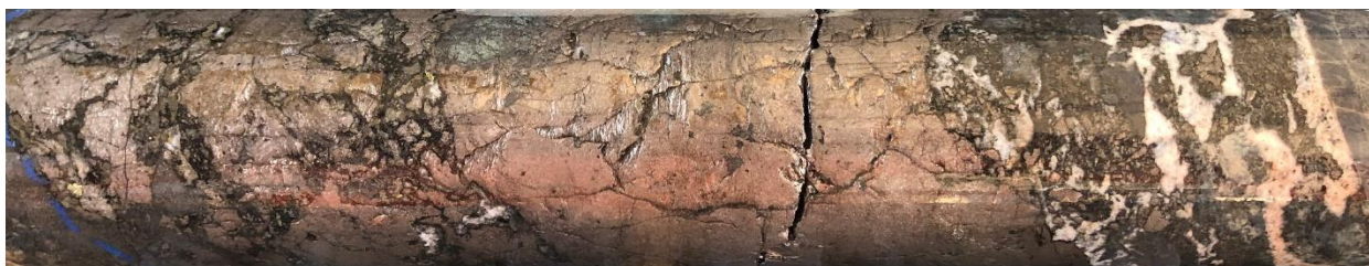
Figure 9. Pyrrhotite massive sulphide zone – HMKPDD002, 109.2m.
