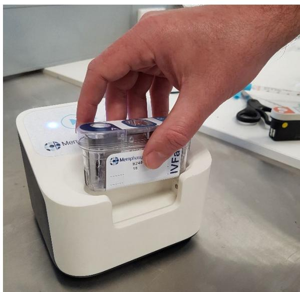
Figure 1: Felix device console and single-use cartridge
