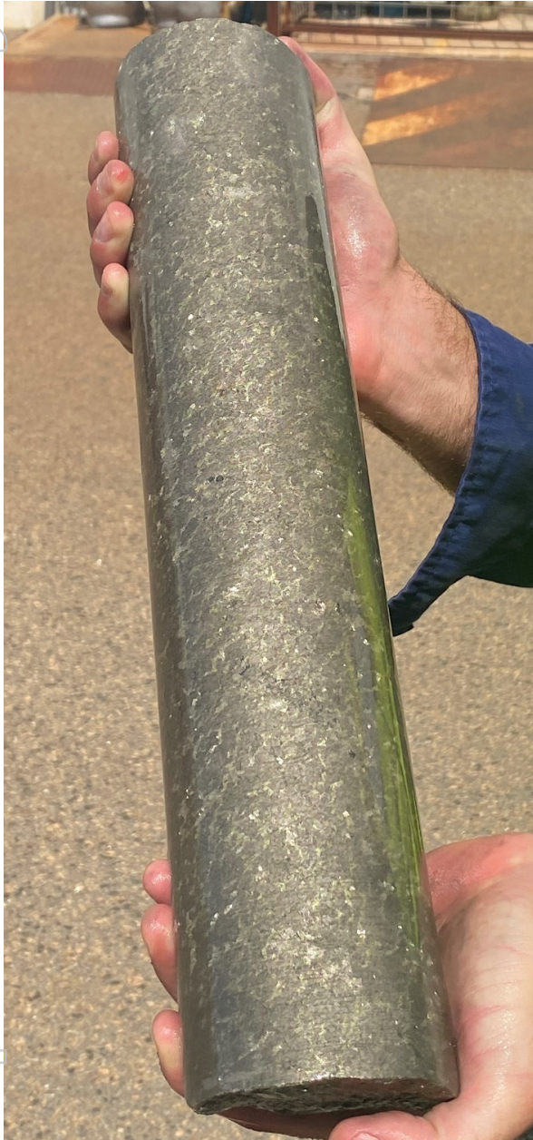
Figure 1 - drill core from MAD177 at approx. 185m downhole showing massive sulphides with coarse grained pentlandite and chalcopyrite.
