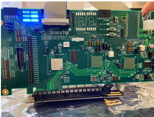
The Akida NSoC neuron fabric is comprised of cores that are organized in groups of four to create nodes, which are mesh networked. The cores can be implemented for either convolutional layers or fully-connected layers. This flexibility allows users to develop networks with ultra-low power Event-Based Convolution as well as Incremental Learning. The nodes also can be used to implement multiple networks on a single device.
