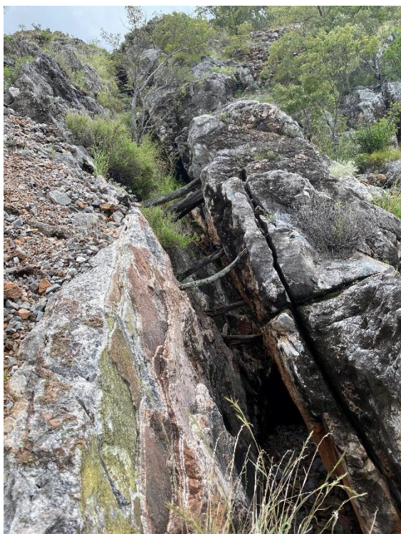
Figure 9: Open stope at Baltika Mine exploiting a laminated vein containing vanadium mineralisation (green mineral).
