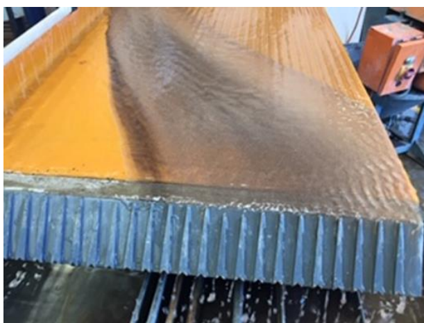
Figure 5: Separation process in action (with noticeable dark hue to the left indicating the presence of descloizite).
