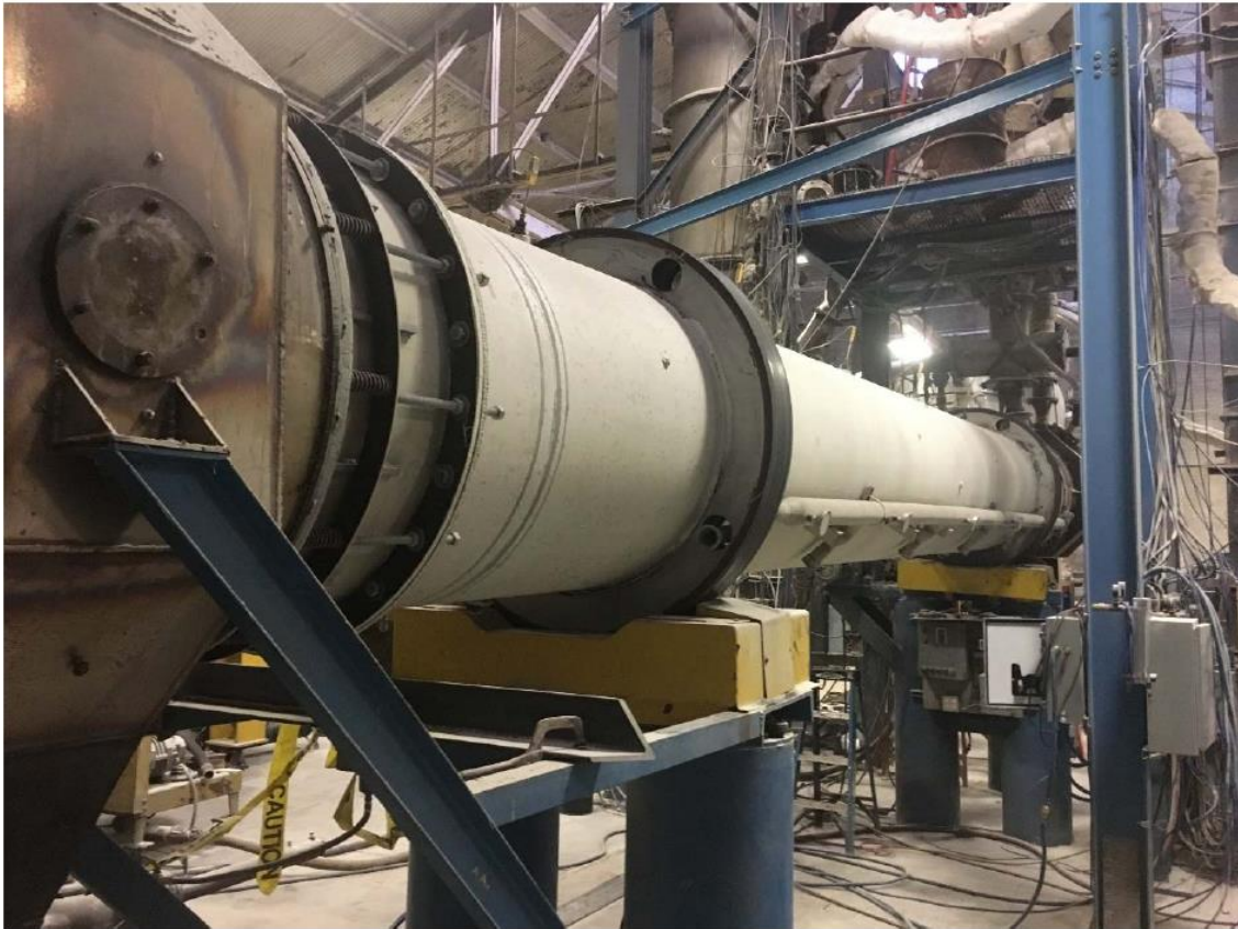
Figure 4: Pilot Rotary Kiln (9.8m long by 0.9m diameter) at FLSMIDTH Test Facility
