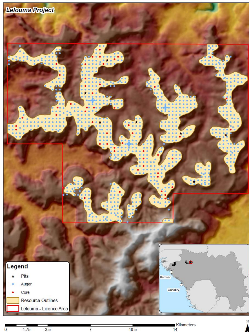
Figure 3 - Drillhole and pit collars coloured by drill type with Lelouma permit boundary (red)
