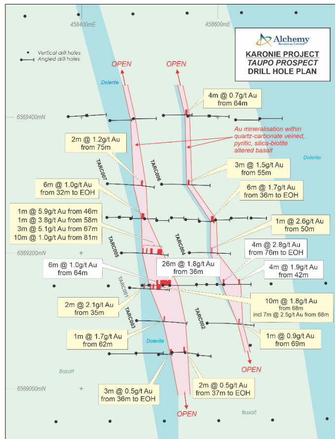
Figure 8: Taupo Prospect: Significant intercepts over interpreted geology (Alchemy intercepts in yellow text boxes)
