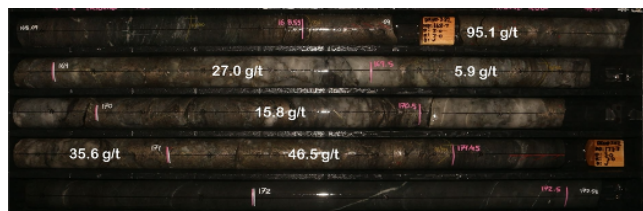
Figure 12: Tribune Lode DRDD382 - Tribune North milky and smokey quartz, hosted in moderate biotite/amphibole shearing. Overall 30% sulphide, locally semi-massive with fracture fill to cataclastic textures, chalcopyrite minor with pyrrhotite dominant +35 flecks of gold logged. Interval assayed 2.9m @ 36.5g/t gold (ASX 18/2/20). 2
