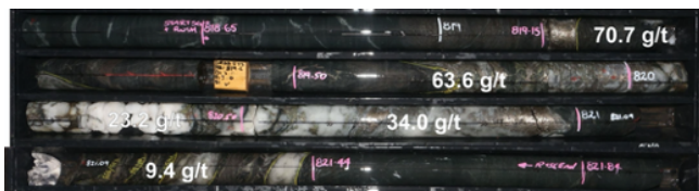
Figure 15: SOUTHERN STEP OUT diamond drill core from DRDD273, high-grade lode mineralization confirmed at the new DHEM plate at the southern extent of the currently tested strike of Deacon; 10% pyrrhotite, trace chalcopyrite and trace visible gold mineralization.
