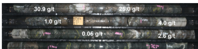
Figure 9: Northern Deacon diamond drill core from DRDD313, drill hole confirms high-grade mineralization associated with the DHEM plates to the north, 5% pyrrhotite, trace chalcopyrite and trace visible gold mineralization. Drill hole is outside current resource area. Interval assayed 3.0m @ 12.0g/t gold (ASX 17/12/19). 2
