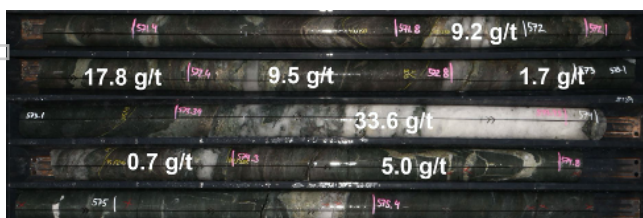
Figure 9: Northern Deacon diamond drill core from DRDD313, drill hole confirms high-grade mineralization associated with the DHEM plates to the north, 5% pyrrhotite, trace chalcopyrite and trace visible gold mineralization. Drill hole is outside current resource area. Interval assayed 3.0m @ 12.0g/t gold (ASX 17/12/19). 2
