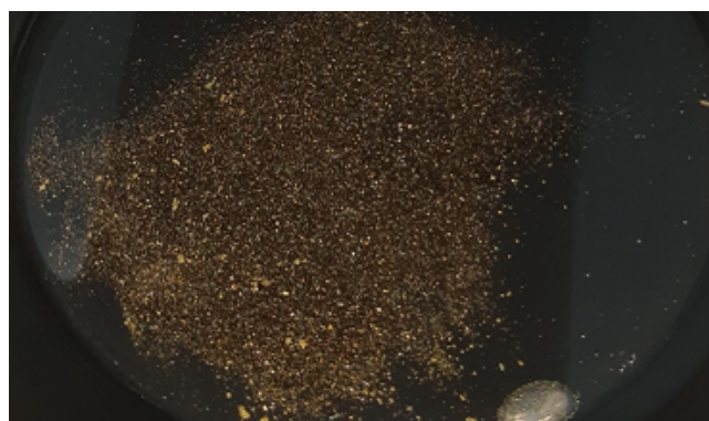
Figure 5: Gravity concentrate recovered from the Viago Lode 10 kg, sample showing abundant gold grains
