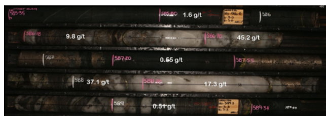
Figure 12: Tribune Lode DRDD382 - Tribune North milky and smokey quartz, hosted in moderate biotite/amphibole shearing. Overall 30% sulphide, locally semi-massive with fracture fill to cataclastic textures, chalcopyrite minor with pyrrhotite dominant +35 flecks of gold logged. Interval assayed 2.9m @ 36.5g/t gold (ASX 18/2/20). 2
