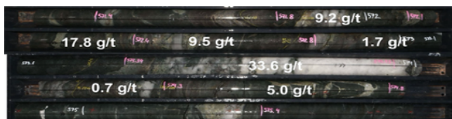
Figure 19: Bellevue South Lode diamond core hole DRDD191 situated above the Viago Lode high-grade mineralization associated with ~5% semi-massive pyrrhotite, trace disseminated chalcopyrite and fine-grained visible gold.
