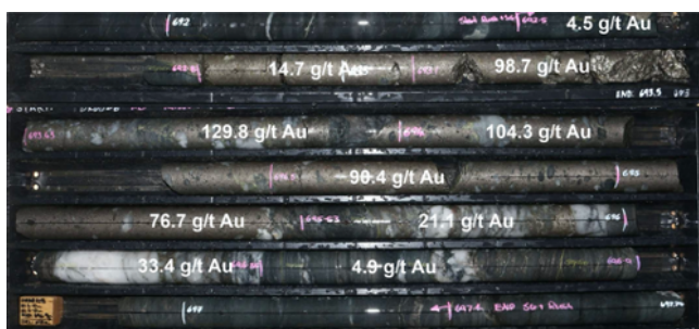
Figure 7: Central Deacon Lode - hole DRDD218 high-grade mineralised shoot with massive pyrrhotite, trace chalcopyrite, quartz clasts and numerous visible gold grains. Interval assayed 4.4m @ 62.4g/t gold from 692m (ASX 10/9/19). 2
