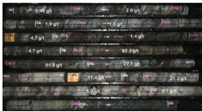
Figure 11: Tribune Lode DRDD360 dominant milky quartz, hosted in moderate biotite/amphibole shearing. Overall 30% sulphide, locally semi-massive with fracture fill to cataclastic textures, chalcopyrite minor with pyrrhotite dominant. Interval assayed 3.2m @ 9.8g/t gold (ASX 18/2/20). 2
