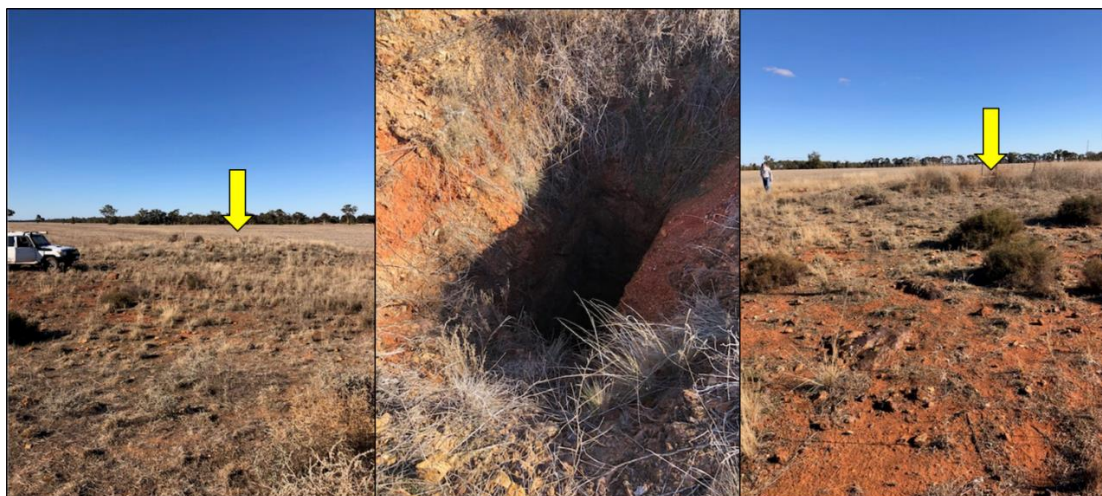
Figure 11: Tindall's Prospect: Yellow arrows define positions in photos of the two +50m deep historic shafts approximately 40m apart (E-W strike). Brecciated Ironstones sub-crops along this trend (similar to Collerina Deposit) - foreground of third photo.
