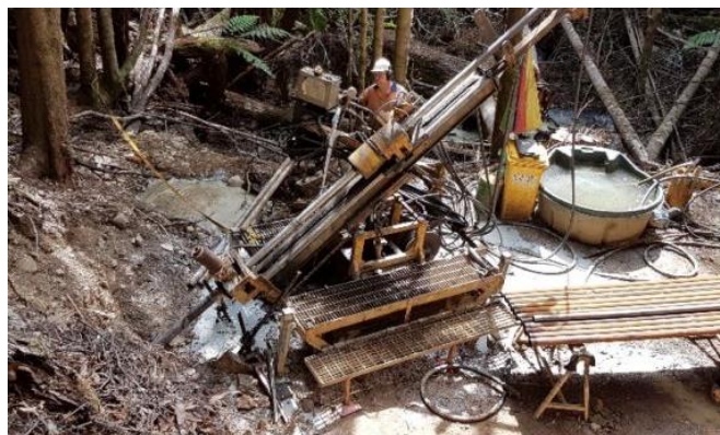
Diamond Drilling at Cleveland 2018
