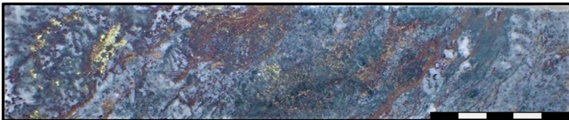
Picture 1: Drill core from KIODD004 (127m) – chlorite-actinolite-pyrrhotite-sphalerite-chalcopyrite-quartz-carbonate-epidote zone
