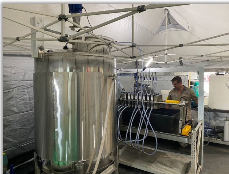
Demonstration scale pre-cursor circuit generated 99.998% purity HPA
