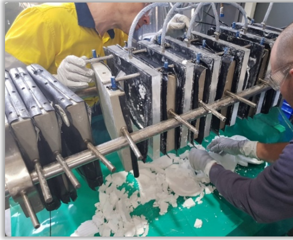
Removal of HPA pre-cursor from the filter
