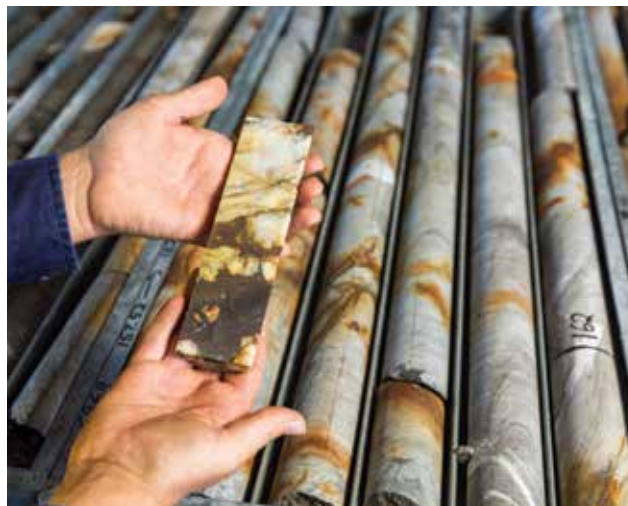
Drill core with wolframite mineralisation
