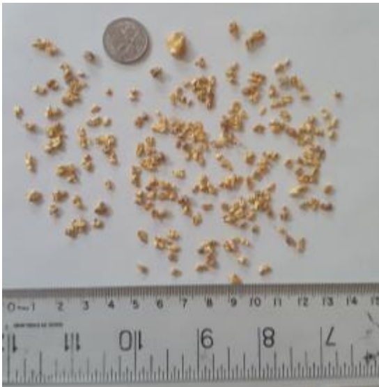
Fig 3 Photographs of the gold nuggets being recovered from the core of the Top Camp area (216 nuggets for 36 grams) and an example of a gold particle intergrown with laminated vein consisting of a core of iron-oxide and a margin of lighter coloured quartz and carbonate (photos are provided by P Gower and the gold is not the property of CZR Resources Ltd).
