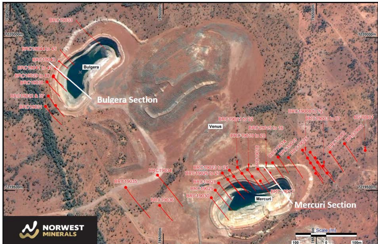
Figure 2 – Bulgera gold project - reverse circulation (RC) drill collar and section locations (figures 3 & 4 below).
