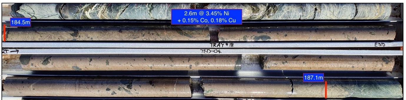
Figure 5: Photo of massive nickel sulphide intersection in diamond hole TED04, the Dusty nickel discovery.
