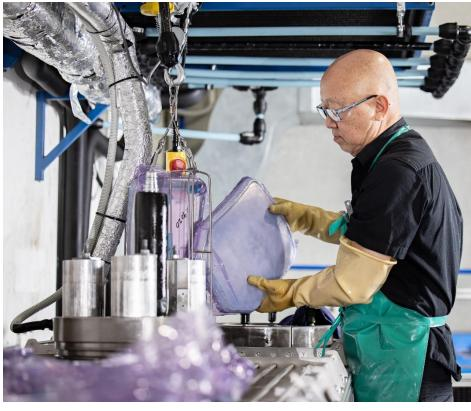
The XTclave is an **advanced composite materials curing and consolidation technology,** that uses ultra-high isostatic pressure at elevated temperatures
