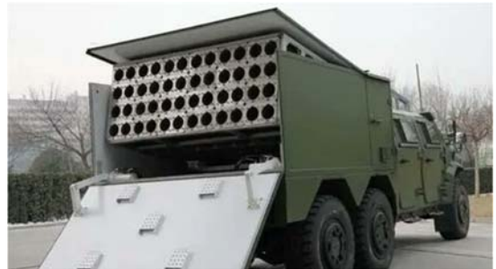
Image: A Chinese UAS/drone fires from a launcher mounted to a Dongfeng Mengshi light tactical vehicle
