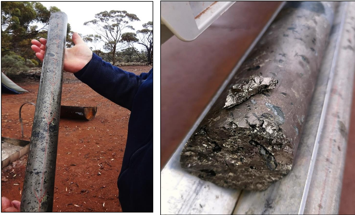
Figure 1. Ni-Cu bearing massive sulphide zone in diamond drill hole CBDD030 drilled 300m south of the T5 Ni-Cu discovery zone (436.7m-437.6m shown).
