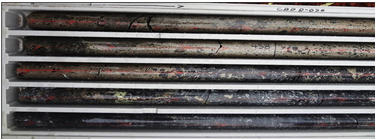
Figure 2. Unique magmatic sulphide textures showing breccia rip up clasts within the massive sulphide, interstitial sulphide/crystal intergrowth at the margin, and chalcopyrite segregation within the crystallised host gabbro. Coarse blebs of matrix sulphide are observed between the crystallising host rock (436.7m-441.1m shown).
