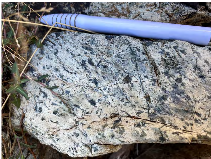
Spring Creek Road Prospect: Sample of chromite mineralised serpentinised ultramafic
