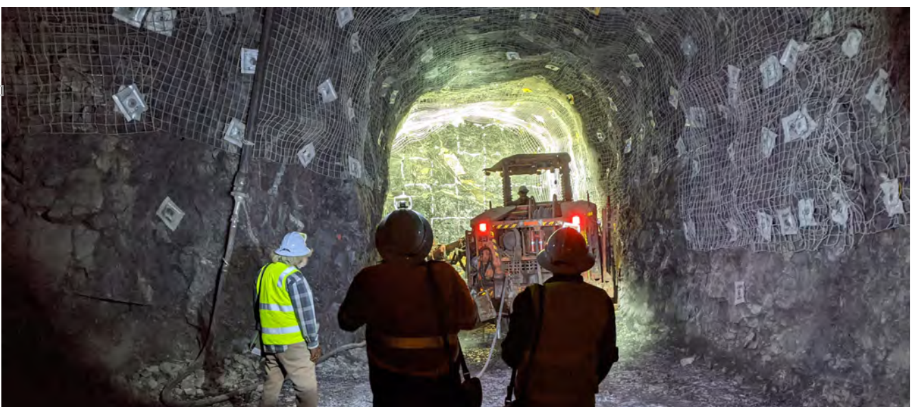
Figure 4: Development Jumbo at the decline face with traditional owners and senior Wati members during a site consultation visit
