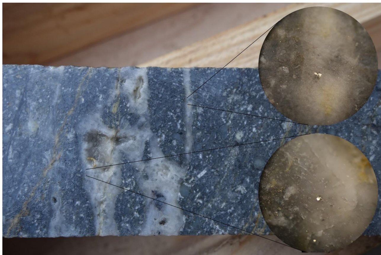
Figure 5: Visible gold associated with pyrite in drusy, fine grained, white chalcedonic quartz at 68.8m in UGA-07
