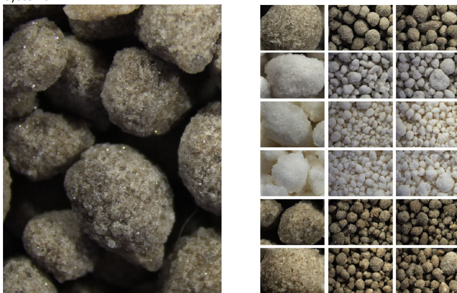
Figure 1: LSOP granulated product showing well-formed granules
