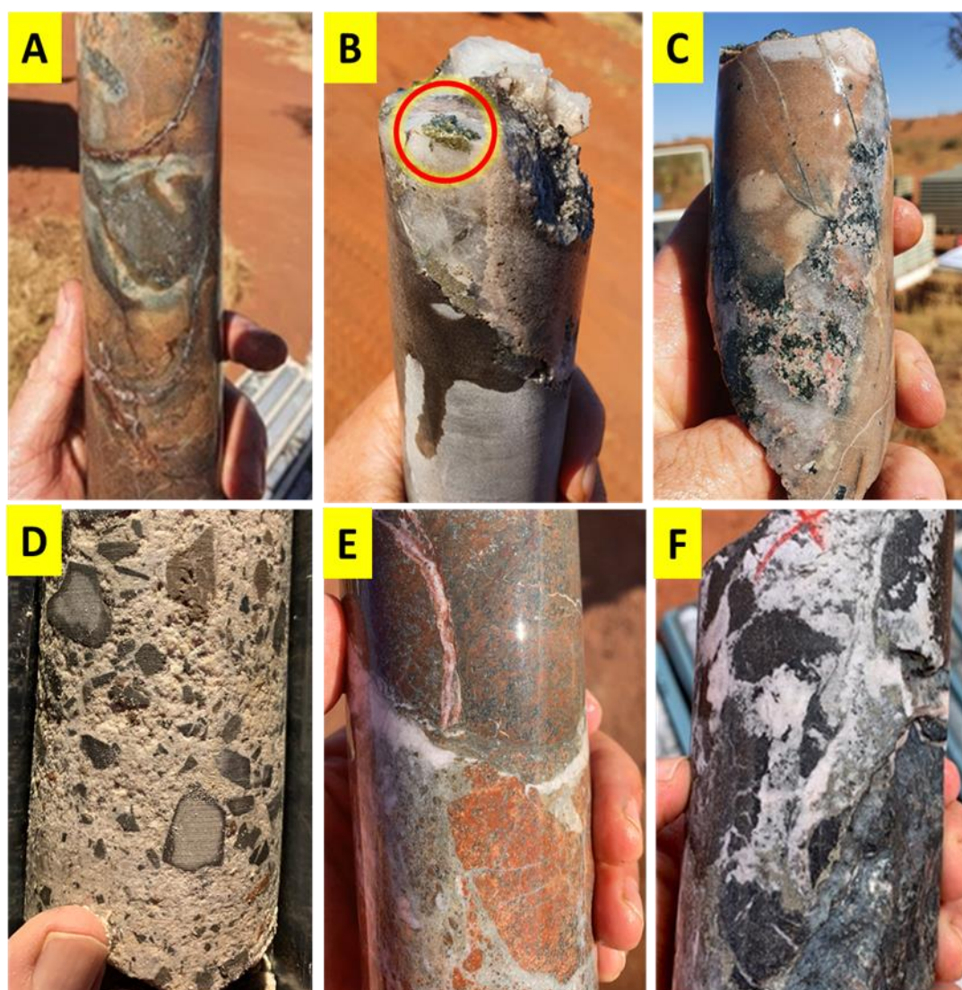
Figure 7: Selected core photographs from Artemis deep diamond holes at the Paterson Nimitz prospect showing zones of hydrothermally altered Proterozoic bedrock and quartz-carbonate-chlorite-hematite veins usually containing trace pyrite and chalcopyrite. A) Hole GDRCD001 from 919m showing carbonate-sericite-hematite altered calcarenite with pyrite and chalcopyrite (<1%). B) Hole GDRCD001 from 1,022m showing calcarenite (bottom) and quartz-carbonate vein (top) with large chalcopyrite mineral grain (inside of red circle). C) Hole GDRCD001 from 972m showing carbonate-hematite altered calcarenite cut by a narrow quartz-carbonate-biotite vein containing trace sulphides (<1%). D) Hole GDRCD003 from 744m showing calcarenite breccia flooded by carbonate-chlorite veining. E) Hole GDRCD003 from 922m showing gabbro highly altered by silica and hematite with trace disseminated sulphides less than 1% (top) in contact with a breccia vein flooded by quartz-carbonate-chlorite and trace sulphides (bottom). F) Hole GDRCD003 from 952m showing brecciated dolerite and quartz-carbonate-biotite-pyrite veining.
