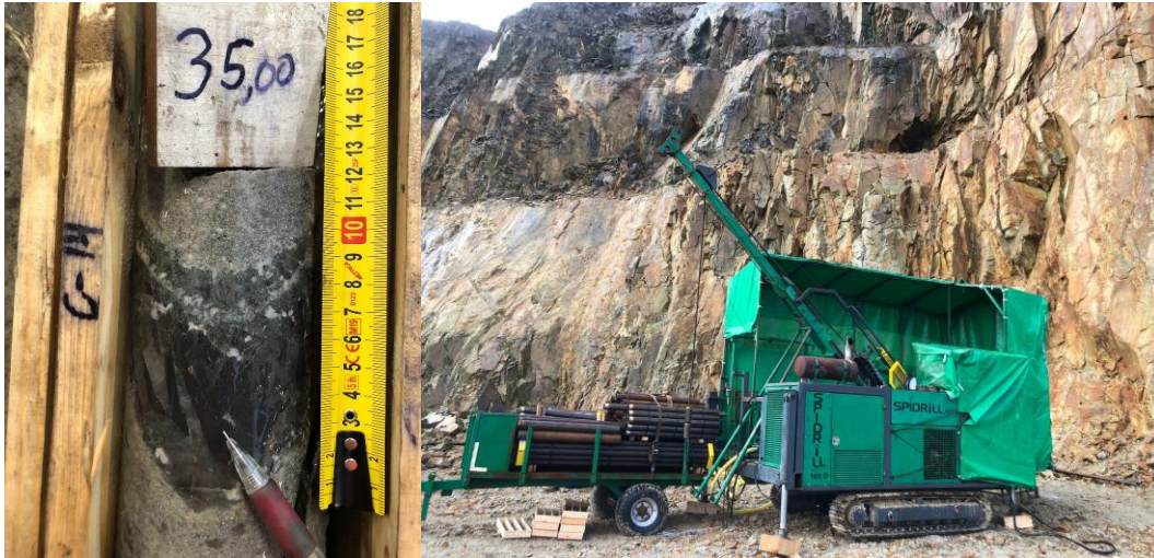
Figures 3 and 4: high-grade wolframite vein (4cm) drill hole 21DD0001 and 2 nd diamond drill rig Spidrill 160D
