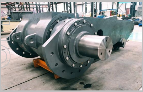
Figure 13 | Trial Assembly of Mill Feed Conveyor
