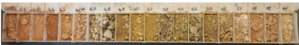
Photo 2: Hole NMWBRC20-101. 45m-50m. 5m @ 5.88g/t Au, incl. 3m @ 9.28g/t Au (45m-48m) Mineralisation associated with quartz / limonite / goethite alteration
