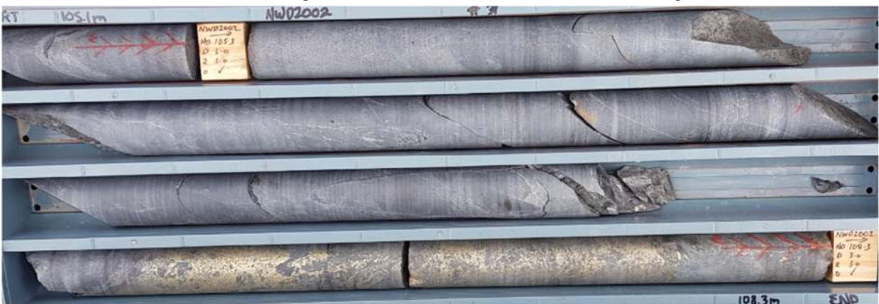
Image 5 | NWD2002 (drill core 107.5m to 108.0m downhole showing chalcopyrite and pyrrhotite mineralisation
