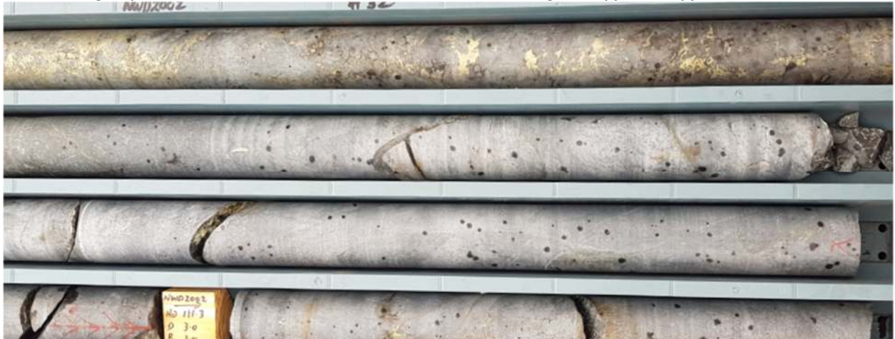
Image 6 | NWD2002 drill core 108.0m to 108.8m downhole showing chalcopyrite and pyrrhotite mineralisation
