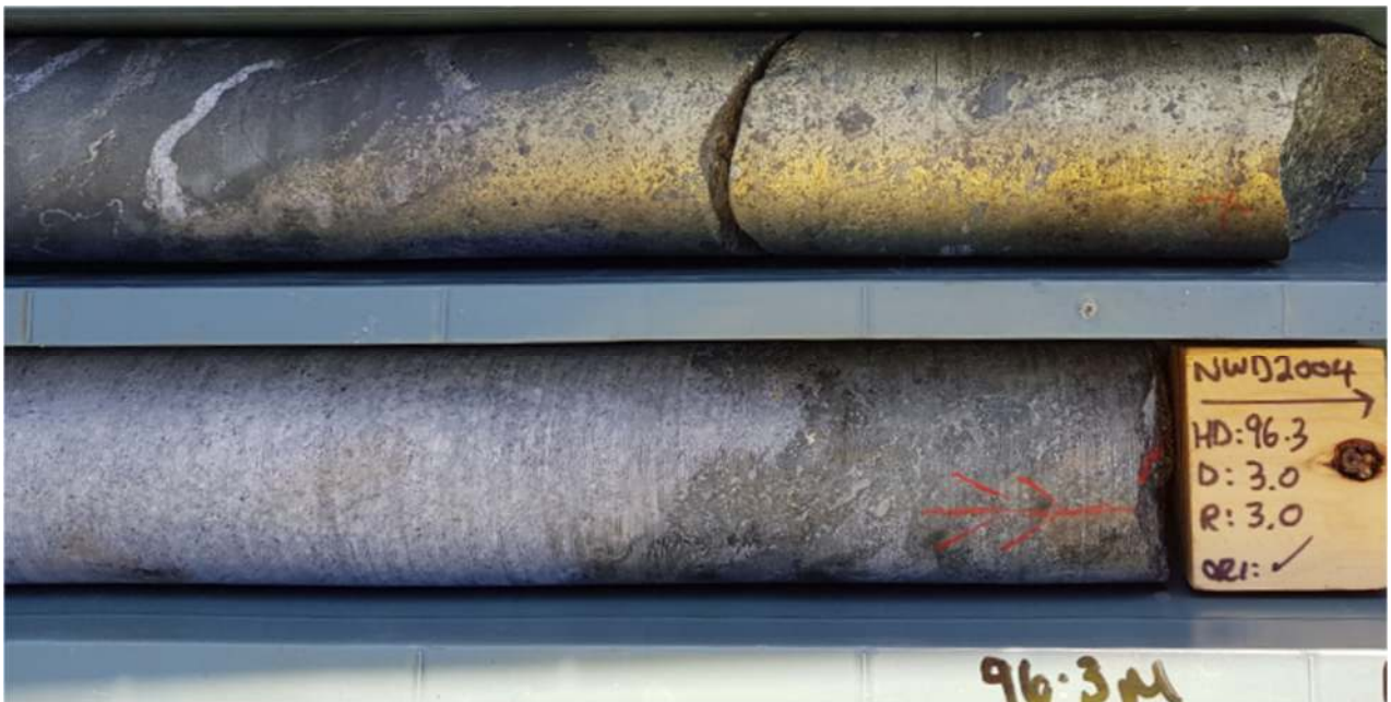
Image 8 | NWD2004 drill core 92.5m to 96.3m downhole showing chalcopyrite copper sulphide mineralisation
