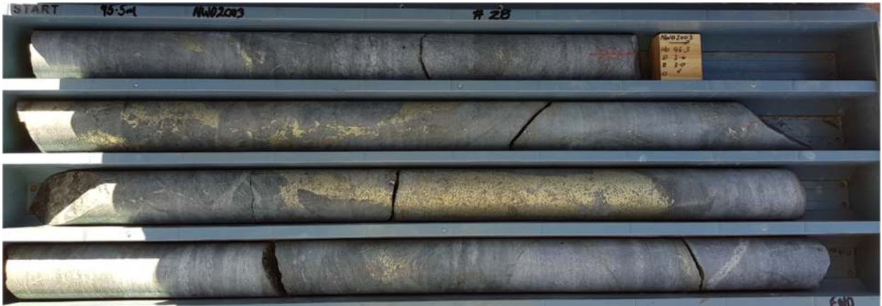
Image 7 | NWD2003 drill core 95.5m to 99.0m downhole showing chalcopyrite and pyrrhotite mineralisation
