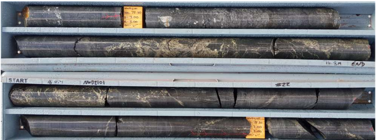
Image 9 | NWD2101 drill core 75.3m to 78.3m downhole showing chalcopyrite and pyrrhotite mineralisation
