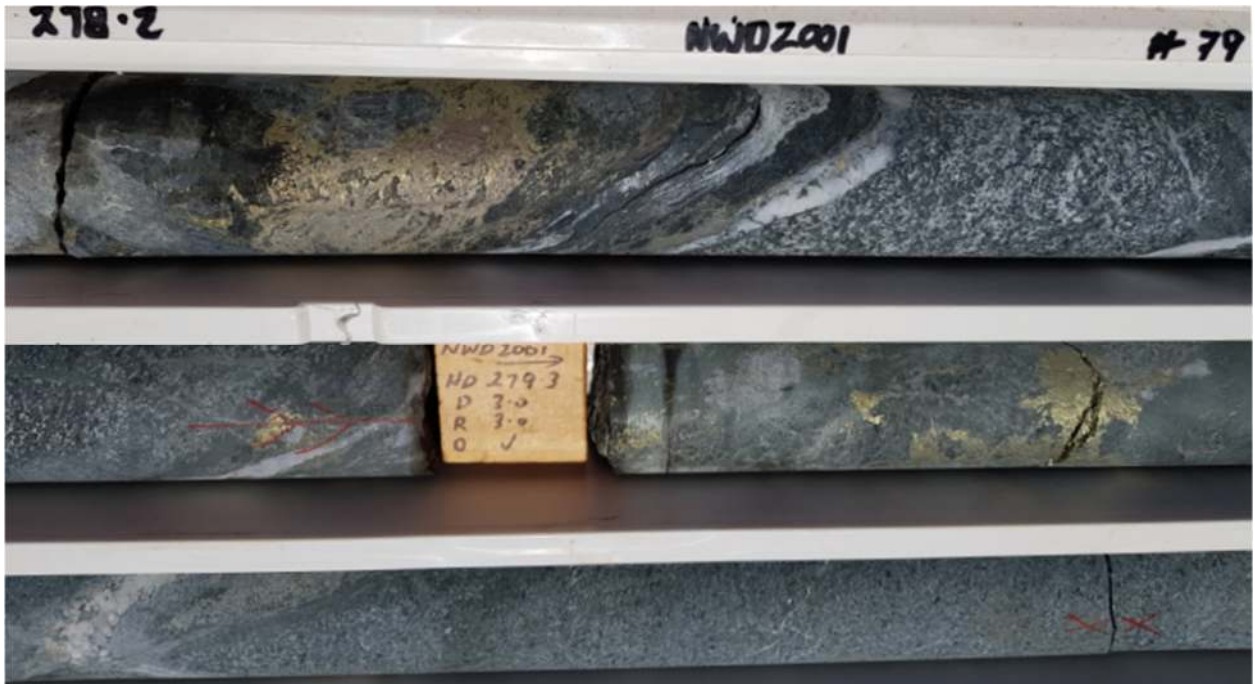
Image 4 | NWD2001 drill core 278.2m to 279.3m downhole showing chalcopyrite and pyrrhotite mineralisation
