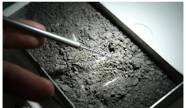
Wellsite geologist examining drill cuttings at Carpentaria-1
