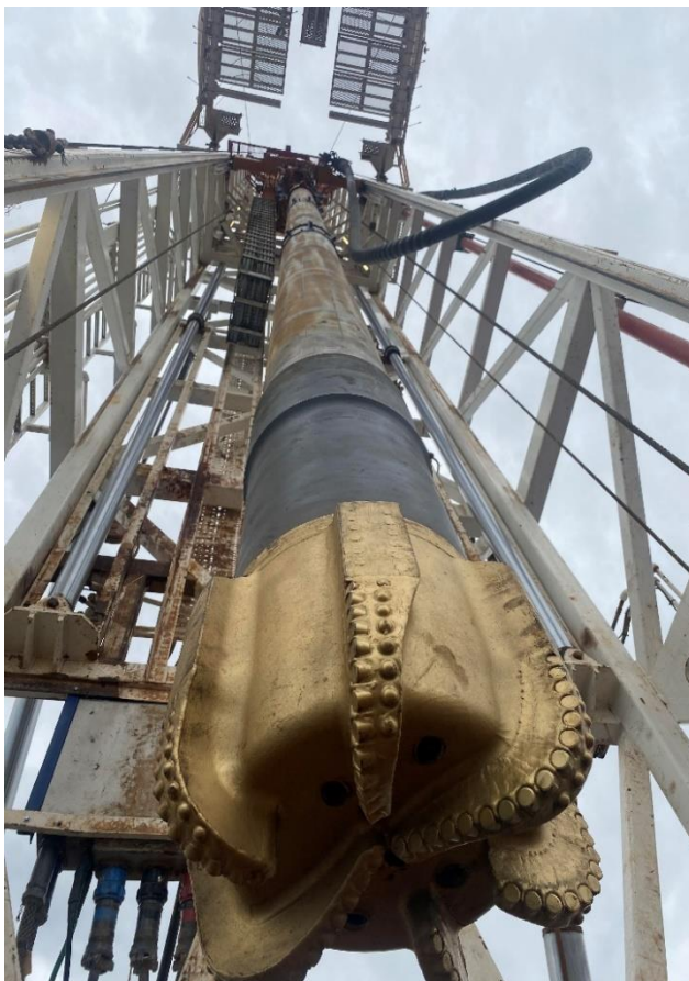
Carpentaria-1 drilling with casing
