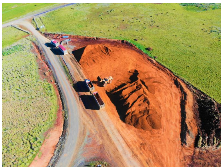
Figure 6 Aerial view of ABx's blending of high-specification cement-grade bauxite by loading trucks from alternate product stockpiles.
