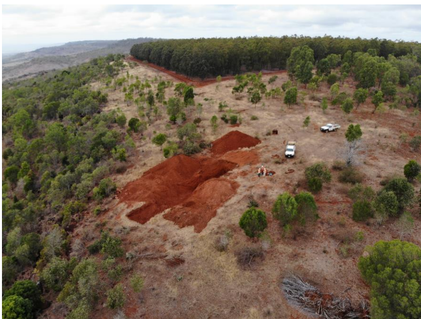
Figure 11: Bulk sample test site Bulk sampling & processing tested the main production parameters. Grades: Results showed that Sunrise Bauxite Project can meet the required marketable grades. Operations: Dust, noise and rehabilitation options were assessed. Rehabilitation: ABx has a post-mining rehabilitation plan to leave the land better than we found it. Bulk dry-screening of a 28 tonne bulk sample satisfactorily tested methods that are expected to be used during production.
