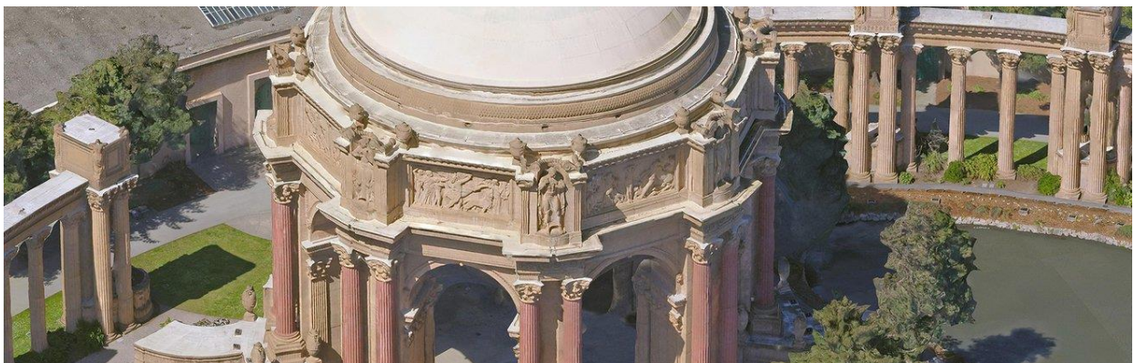
Aerometrex 3D model: San Francisco Palace of Fine Arts. 2cm pixel resolution
