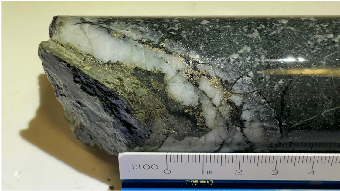
Figure 12 Hydrothermally mobilised chalcopyrite within MIDD007 from 165.0m downhole.
