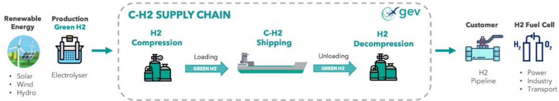
Figure 5: C-H2 Supply Chain Developed by GEV
