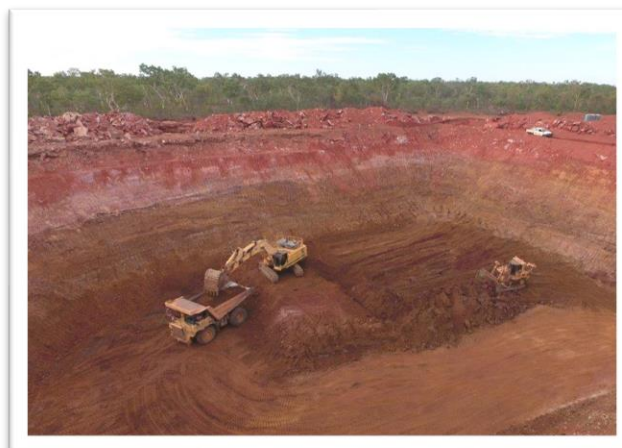
Figure 3: Ore mining by dozer push to fixed excavator location
