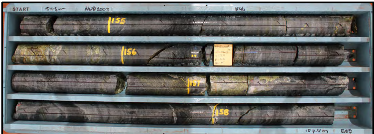
Image 7 | NWD2003: 155.0m to 156.0m; 1.0m @ 5.11% Cu, 0.40 Au g/t and 8.50 g/t Ag. 156.7m to 157.4m; 1.0m @ 11.0% Cu, 0.82 Au g/t and 18.5 g/t Ag
