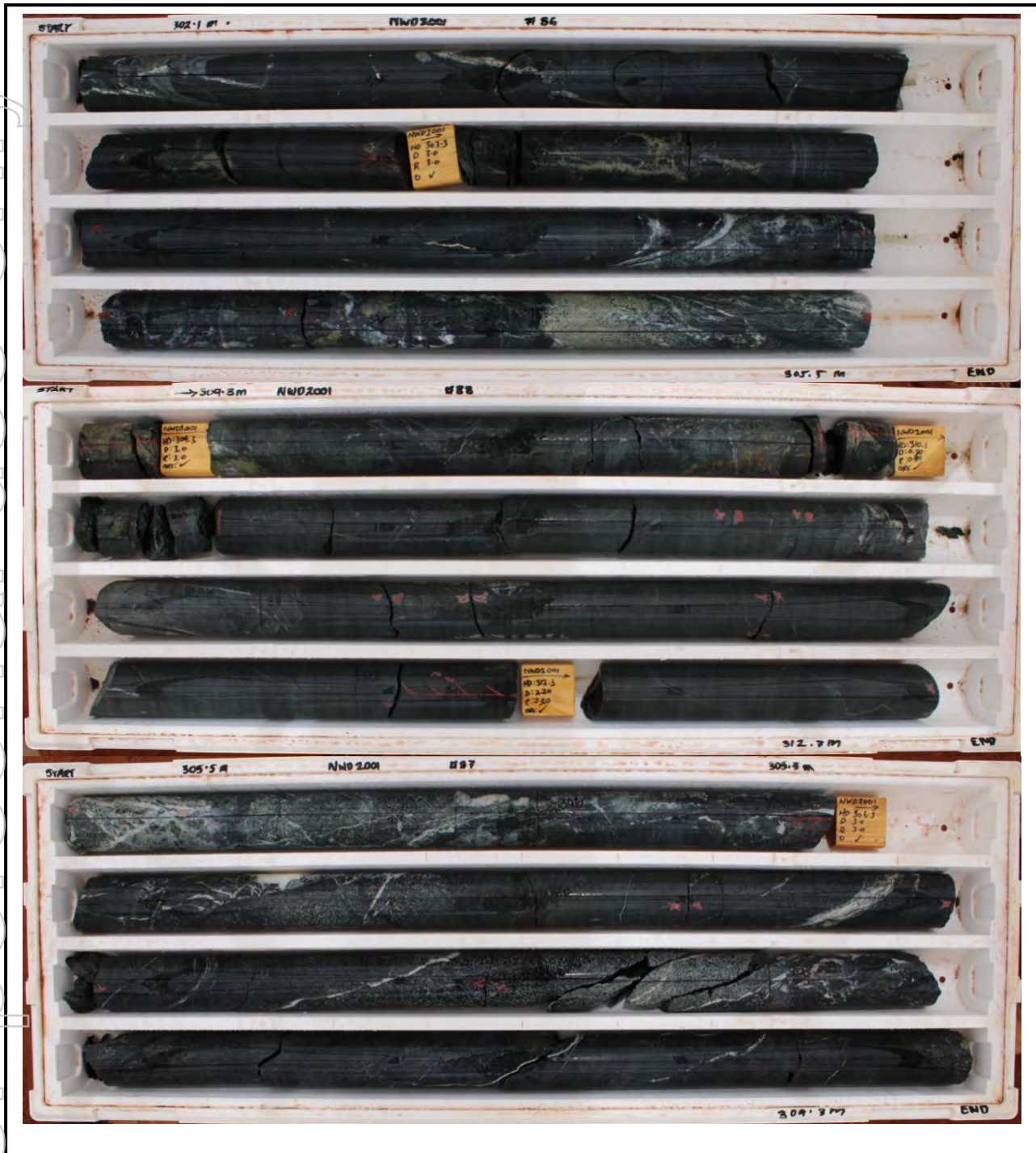
Image 9 | NWD2001: 303.0m to 312.0m; 9.0m @ 392 Ag g/t crackle breccia silver sulphide mineralisation, including 2.0m @ 1,470 Ag g/t from 306.0m.
