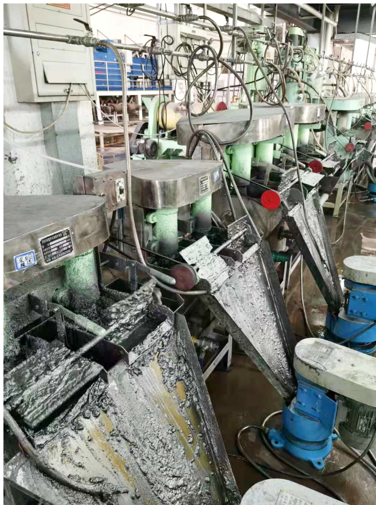
Flotation Circuit used at testing facility
