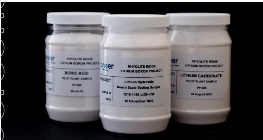
Below: Lithium Hydroxide, Lithium Carbonate and Boric Acid end products produced in the Pilot Plant.
