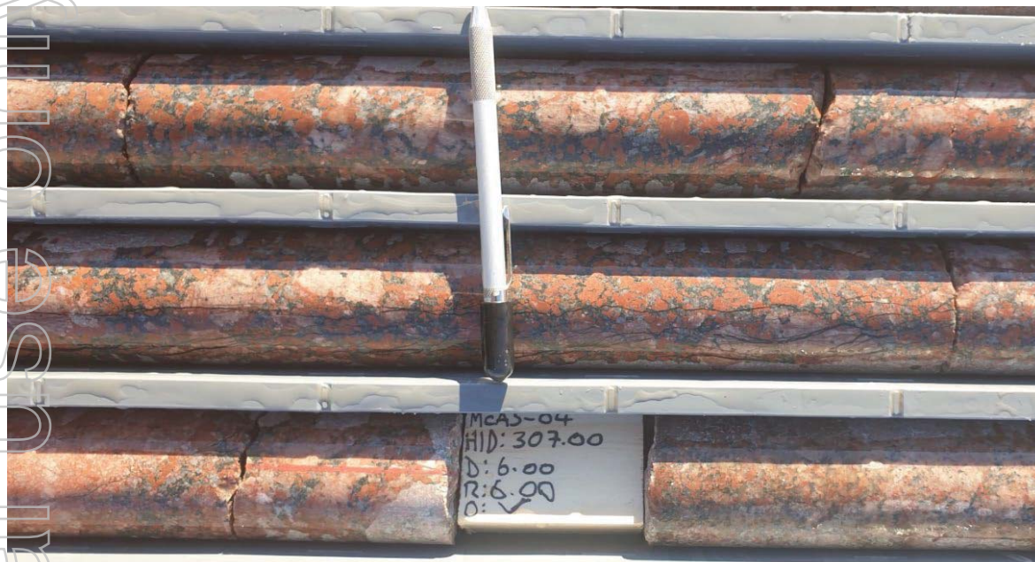
Figure 3 – Hole ID MCDA5-04 – Photo of core tray box 35, showing pervasive Red Rock (silica – hematized K-Feldspar (brick red)) alteration of original porphyritic granite host rock. Matrix of granite is enriched in the light rare earths, cerium, and lanthanum.
