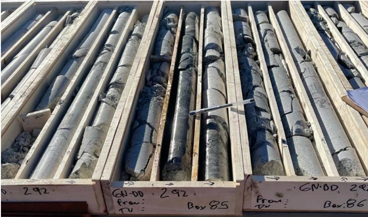
Photo 3 : GNDD-292 sulphide interval 233 metres downhole (skarn alteration 15% pyrite 5% sphalerite)
