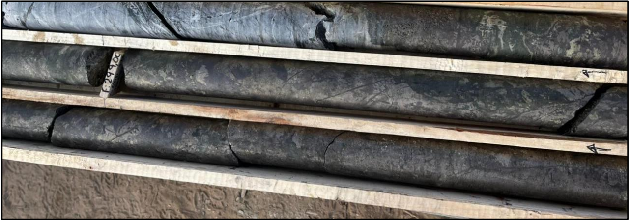
Photo 8 - GNDD-314 Footwall Zone mineralisation from 297-300 metres (2.8m at 62.5 g/t AuEq)
