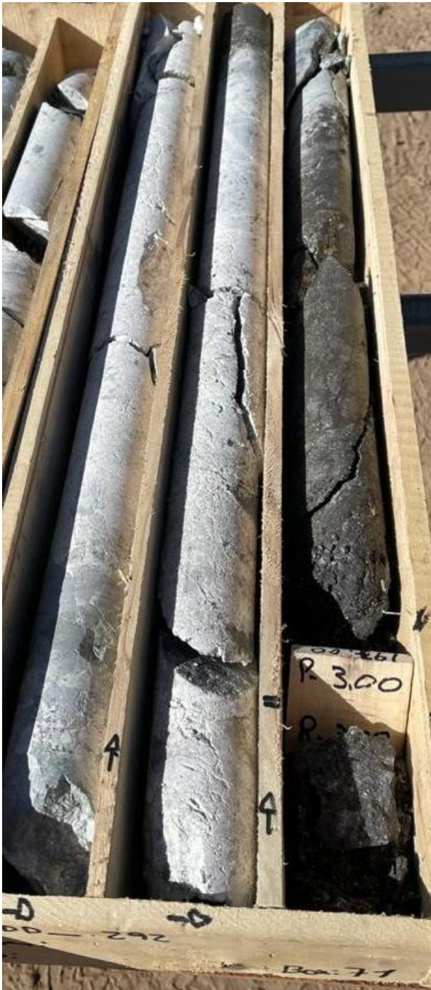
GNDD-292 - sulphide Interval 197-198m
