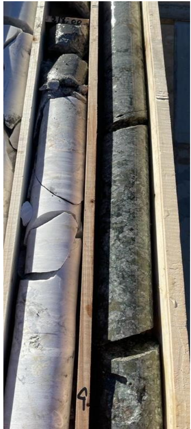
GNDD-292 - sulphide Interval 218-219m
